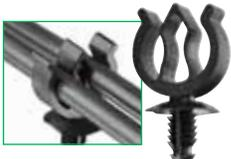
**Helios UVX Clip** (Installs into a .260" mounting hole and holds up to 2 cables between .230 - .315" each).
