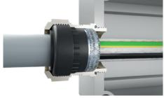
**9** Tighten compression nut to the lower part until the sealing insert bulges slightly between the compression nut and the cable. Please refer to the instruction sheet with details of installation torques on our website, Heyco.com
