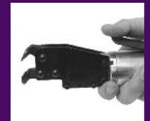
4-29 Original Strain Relief Bushing Air Tool
