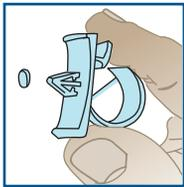
Simply insert base of clip into .250" diameter hole.
